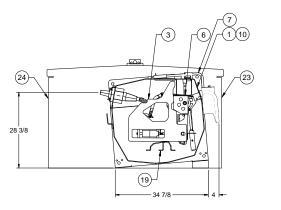
SECTION B-B: FAULT-INTERRUPTER
