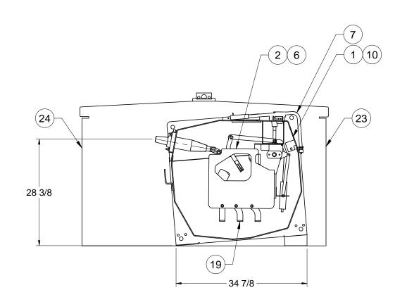
**SECTION A-A: LOAD SWITCH**
